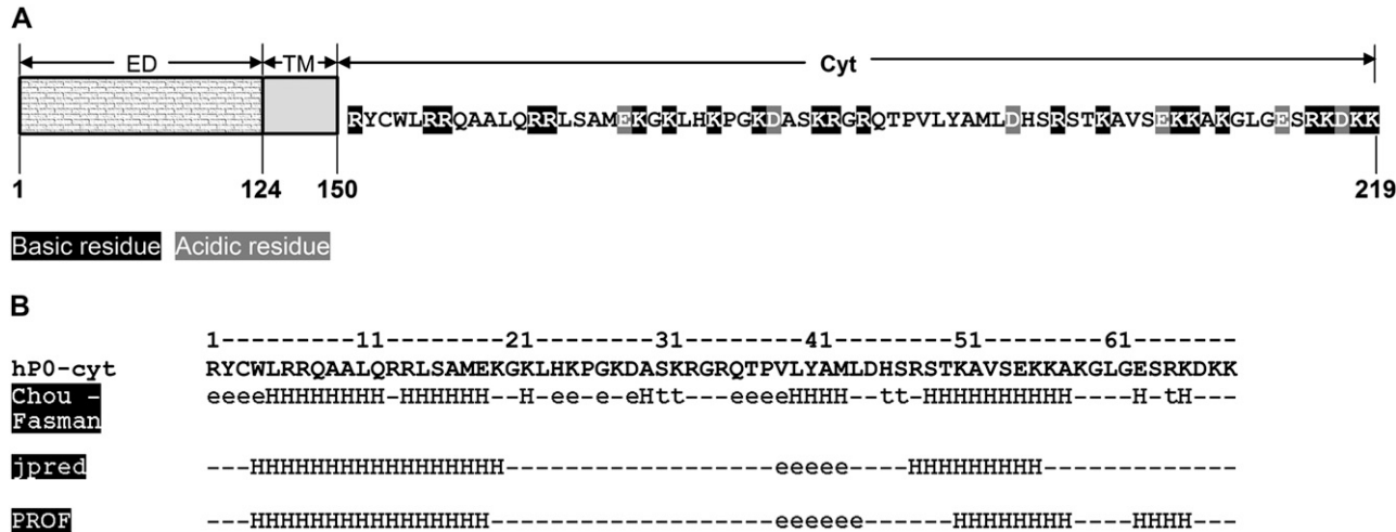
FIGURE 1 Sequence of hP0-cyt (A) and its secondary structure (B) predicted according to Chou-Fasman, JPred, and PROF (19–21). ED, P0 extracellular domain; TM, P0 transmembrane domain; Cyt, P0 cytoplasmic domain. hP0-cyt contains 69 residues (151–219) and is highly basic, with a net charge of +15, pI = 10.88 . H, \alpha -helix; e, \beta -strand; t, turns.
